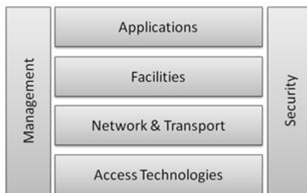
Figure 4-25. Layers of the ITS V2X communication stack
