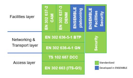
Figure 1 - Security in the V2X communication stack
