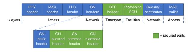
Figure 2 - V2X secured packet
