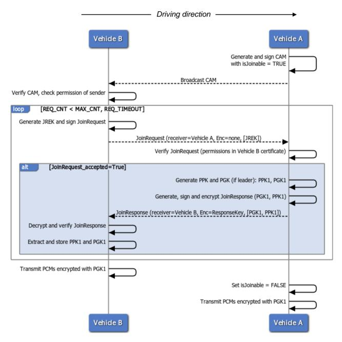
Figure 6 - Key handling at the joining procedure
