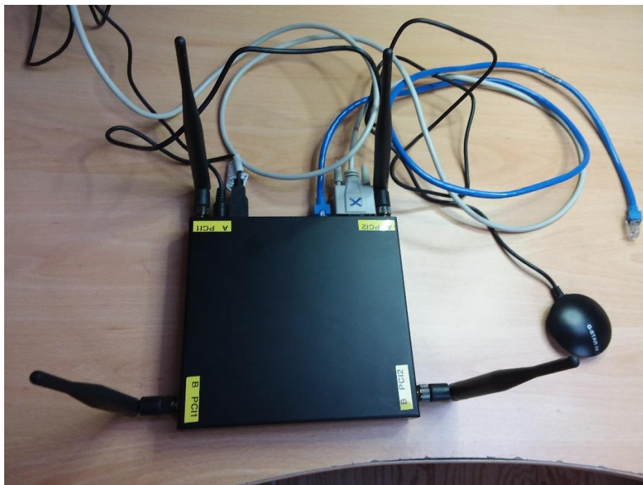
Figure 3: Hardware of the V2X Sub-System (of the ENSEMBLE Reference Implementation).
