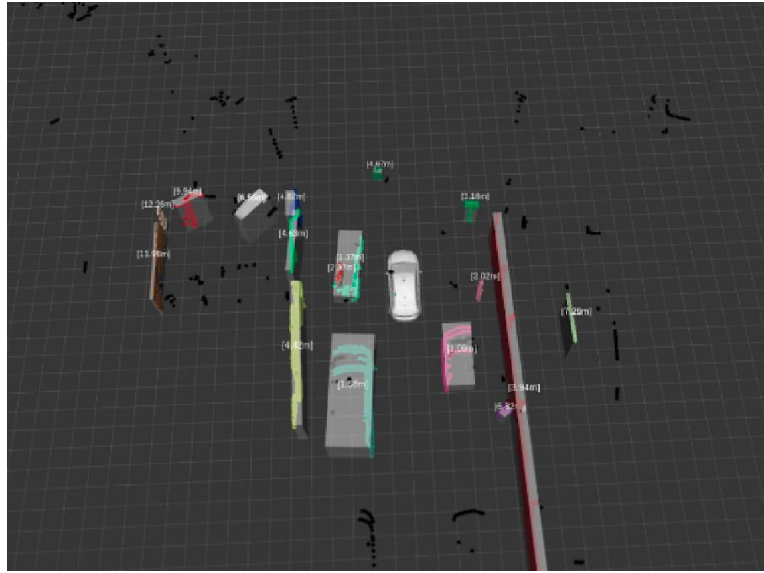
Figure 4 Object detection on point clouds. Top: On the left, each cluster is painted with a different color and the convex hull is displayed in blue, the corresponding bounding boxes are shown in the right image in white. Bottom: All the clusters and bounding boxes detected.
